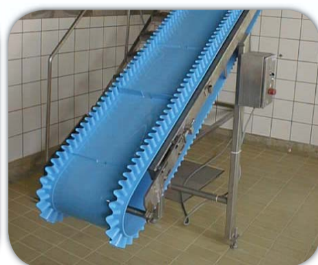
SuperDrive™ with sidewalls & special flights
