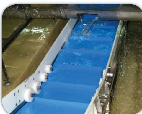
SuperDrive™ with flights working under water
