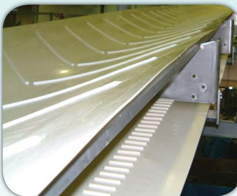
SuperDrive™ Trough Conveyor with Chevron flights
