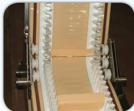
SuperDrive™ Z-elevator with flights, guides and sidewalls
